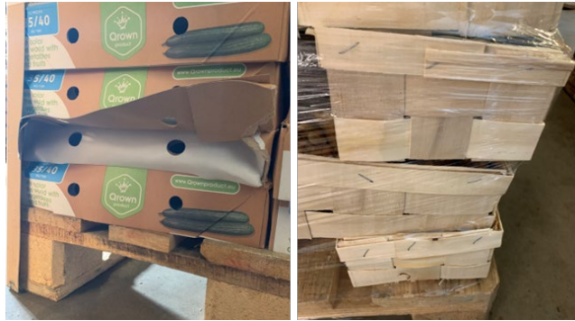
Figure 10: Examples of damage caused by a lack of stability (left) and a lack of modular tuning (right)
