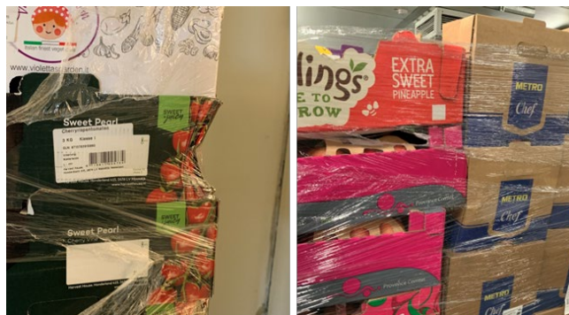
Figure 11: Examples of damage caused by external influences (left) and inadequate loading unit securing (right)
