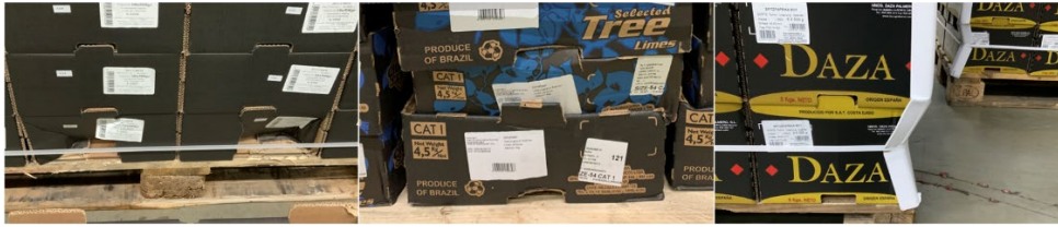
Figure 7: Examples of damage: external influences (left), lack of stability (center), inadequate loading unit securing (right)
